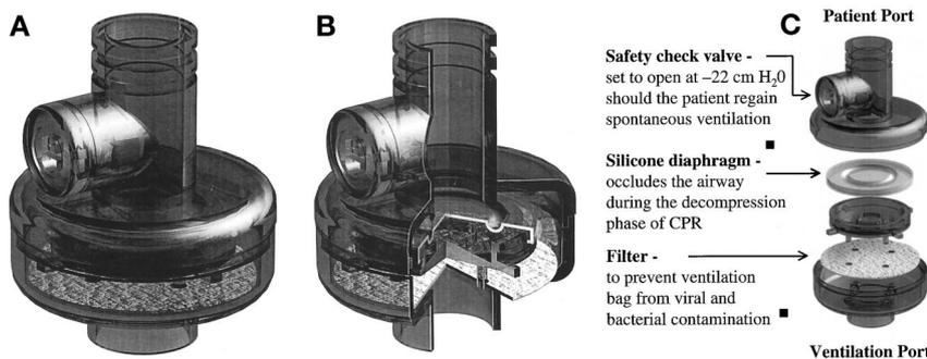
Figure 1. The inspiratory impedance threshold valve (ResQ-Valve, CPRx LLC, Minneapolis, MN) functions by occluding the airway during the decompression phase of cardiopulmonary resuscitation (CPR). The small valve is easily inserted into any standard respiratory circuit between the ventilation bag and endotracheal tube, face mask, Combitube, or laryngeal mask airway. The valve (A) and cut-away views (B and C) are shown.
