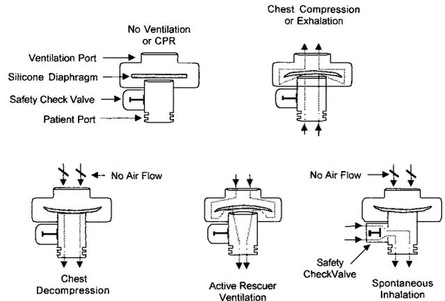
Figure 1. Schematic of respiratory gas flow through ITV.
