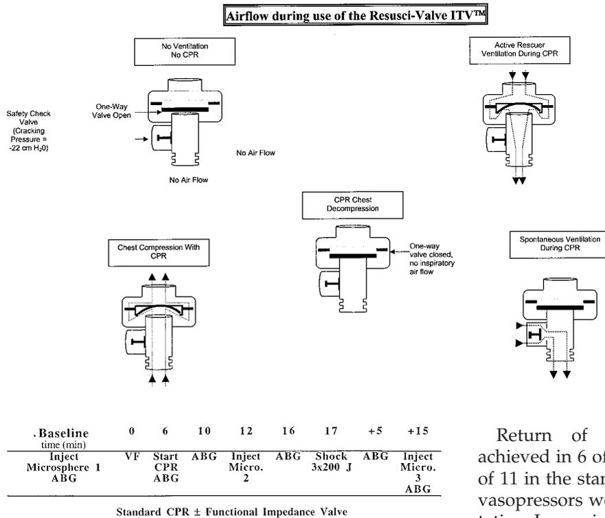
Figure 2. Schematic representation of respiratory gas flow through the impedance valve in the absence and presence of cardiopulmonary resuscitation (CPR). During a spontaneous breath, a safety check valve opens at a cracking pressure of -22 cm H<sub>2</sub>O, enabling inspiration. ITV = impedance threshold valve.
