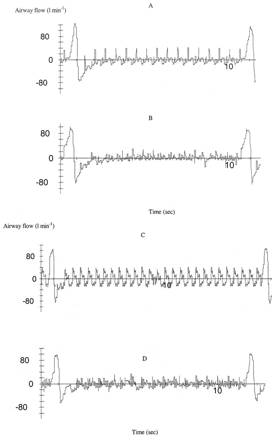
Fig. 1. Airway flow (l min<sup>-1</sup>) generated with standard CPR (A), standard CPR with valve (B), ACD-CPR (C) and ACD-CPR with valve (D). Inspiratory flow is positive deflections. Passive airway flow is shown between two manual ventilations in four different runs. Inspiratory flow is damped when the valve is present (B, D), demonstrating the function of the valve.
